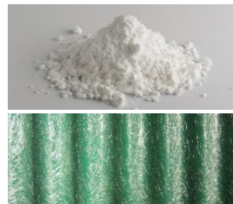
Lart: Mineral mbushes ( \text{CaCO}_3 ) Poshte: Fibra xhami
